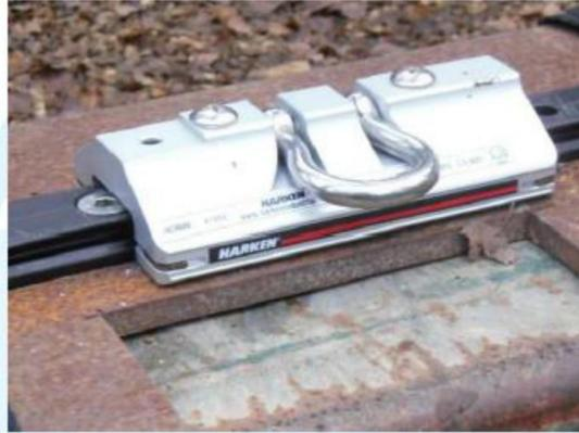
Figure 1 – Anchor device described as “H-49971” in horizontal test direction
