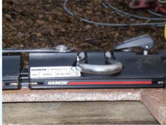
Figure 3 – Anchor device described as “H-49971” in 15° from the horizontal test direction
