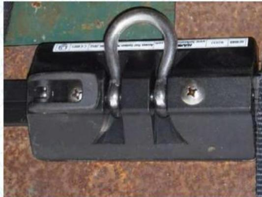
Figure 2 – Anchor device described as “H-49971” in vertical test direction
