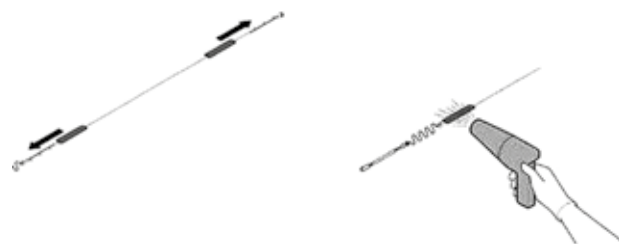
Figure 5.7 - Heating the sheathing
