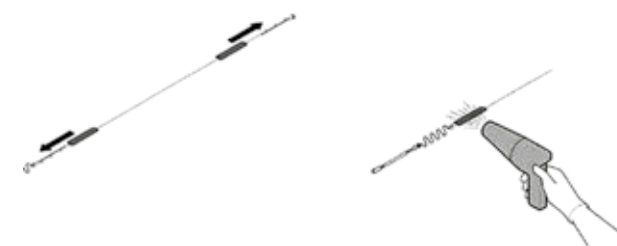
Figure 5.5 - Heating the sheathing
