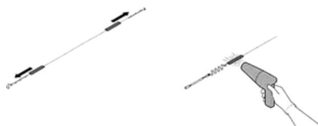
Figure 5.5 - Heating the sheathing
